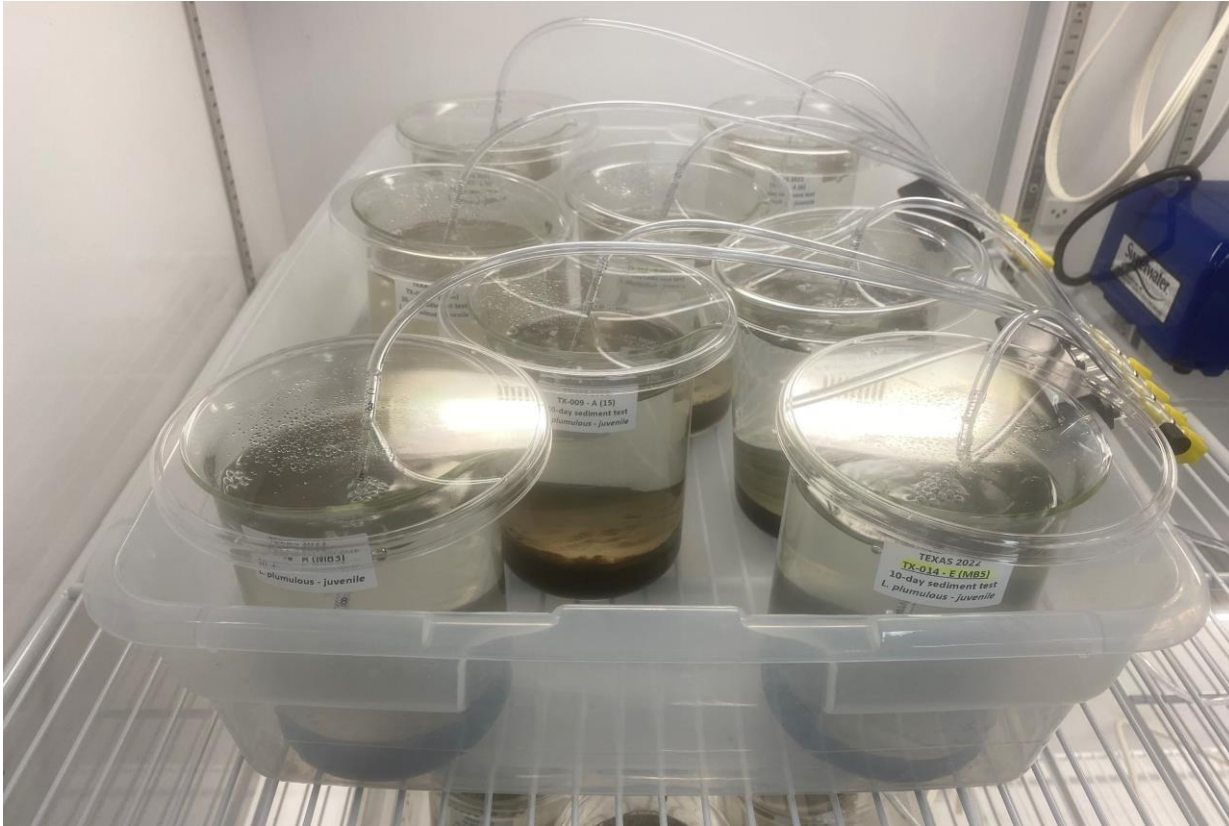
Whole-Sediment Toxicity Test – Expose to sediment
